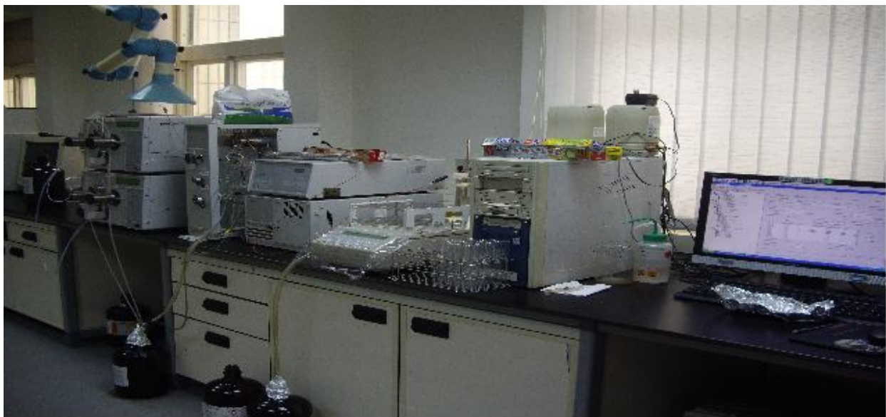
製備型Varian HPLC Prepstar MODEL SD-1
